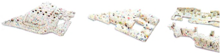
Fig. 4.11 Complex shaped parts from recycled PUR foam.
