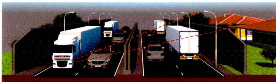
Fig. 6.3 Applied noise reduction wall between two traffic lanes to improve protection
