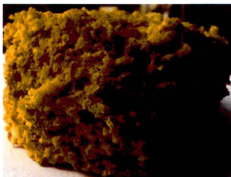
Fig. 4.20 Non-compliant moulding under inappropriate process conditions (150 °C; 2.0 MPa; 12 min endurance).
