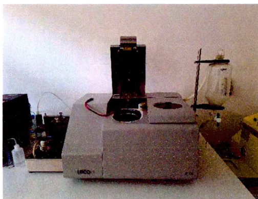
Fig. 8.9 LECO AC500 calorimetric instrument for measuring calorific value of fuels
