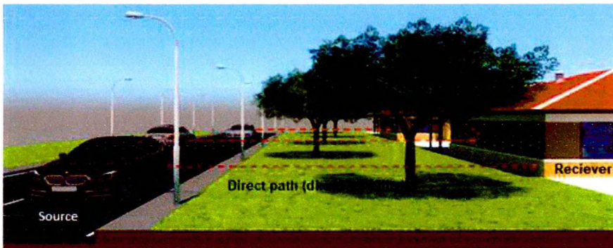
Fig. 6.5 Direction of propagation of sound waves without a reflective noise reduction wall
