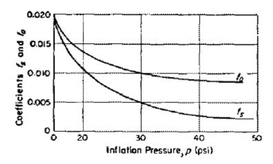
An empirical relationship can be used for speeds up to 130 km/h and a pressure of 26 psi:
