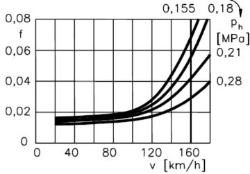
Dependence of rolling resistance coefficient on vehicle speed and tire inflation
