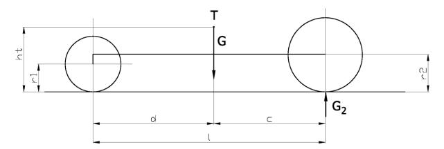
If we know the weight of the vehicle and the vertical force from the rear wheel, then from the condition of moment balance to the axis  $O_1$  we can write:
