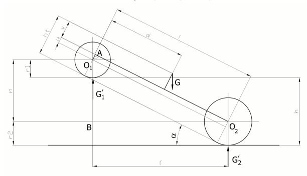
We write the condition of the moment-to-point balance  $O_1$ :
