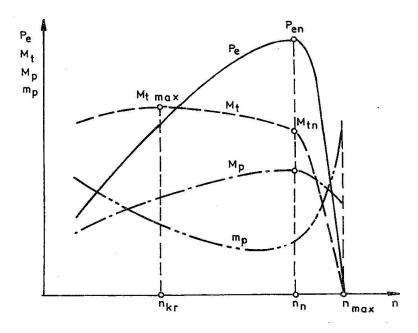
The speed at which the motor reaches the maximum effective power  $P_{en}$  is called the nominal engine speed  $n_n$ . At this speed, the controller allows the maximum fuel supply, which corresponds to the setting of the accelerator lever.
