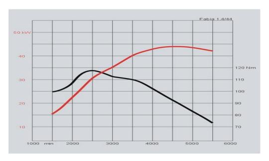
Courses of torque Mk and reduced effective power Pe for the Škoda 1.4 / 44kW MPI engine.
