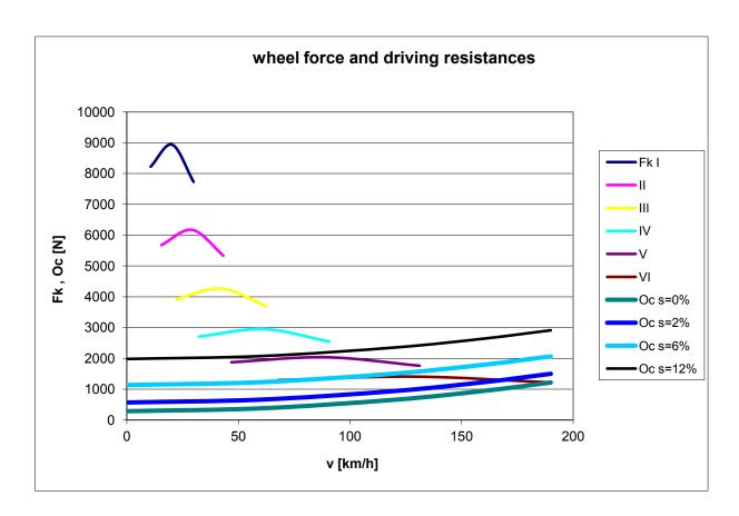
The engine power reserve (the difference between the maximum driving force and the running resistances) can be used for acceleration or as traction at a given constant speed and incline.
